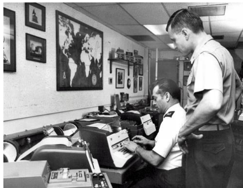
The Hotline terminal room in the NMCC at the Pentagon, 1985 with the new teletype and encryption equipment, installed in 1980.
